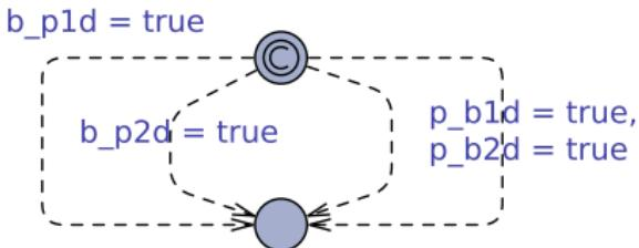
The Defender Automaton for  $D = \{p1d, p2d\}$  with  $A_d = \{p1d, p2d, p3d\}$
